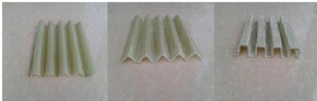
Figure 1. Testing specimens (corrugated composite plates with different profiles sinusoidal, triangular, and square)
