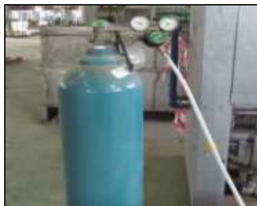
Fig. 2: Argon gas cylinder
