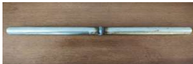
Fig. 4: Illustrate the TIG pipe welding specimen.
