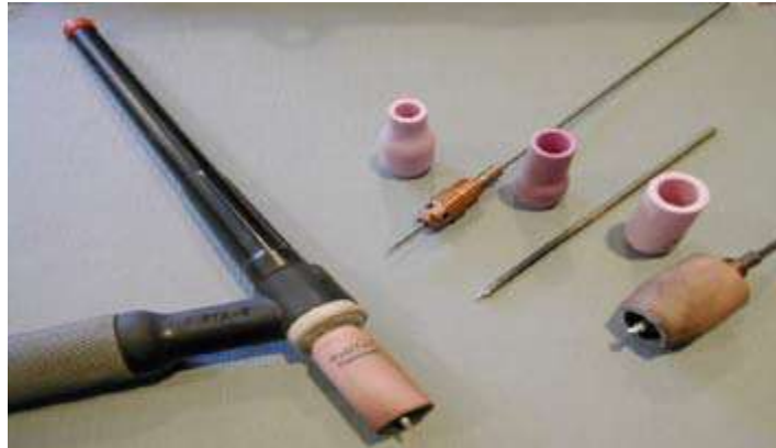
Fig. 3: TIG Welding Torch
