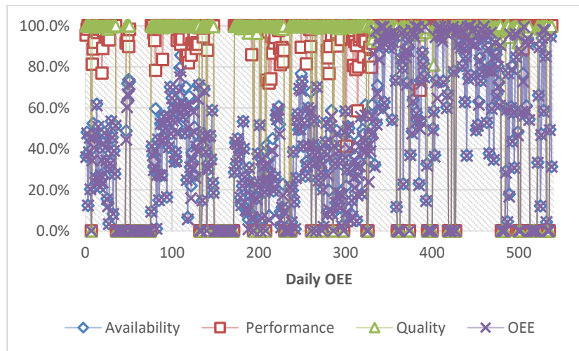
Figure 2. The actual availability, performance and quality rate measures, together with the OEE figure for each day
