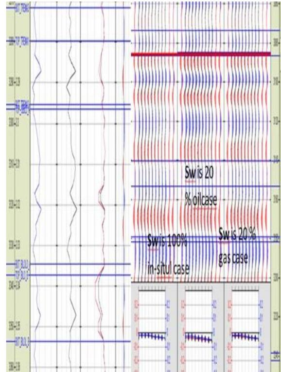
**Figure 7:** shows synthetic AVO modeling for Trema-1 reservoir, one with ricker wavelet of 50 Hz of three cases (in-situ case, gas case, and oil case).
