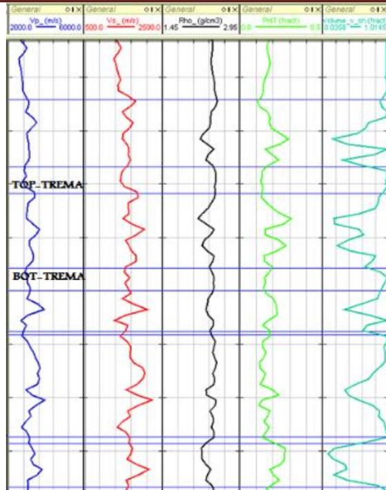
**Figure 5:** shows the elastic parameters logs, and porosity log for Trema-1 well.
