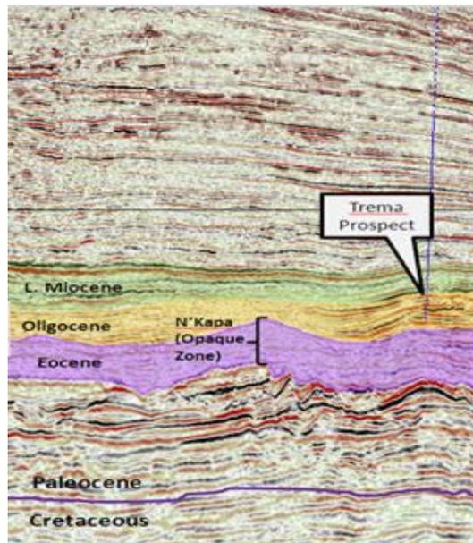
Figure 2: Seismic section through Trema-1 well showing canyon fill sediments in the Tilapia area, west region of Cameroon (Adopted from Noble Energy).
