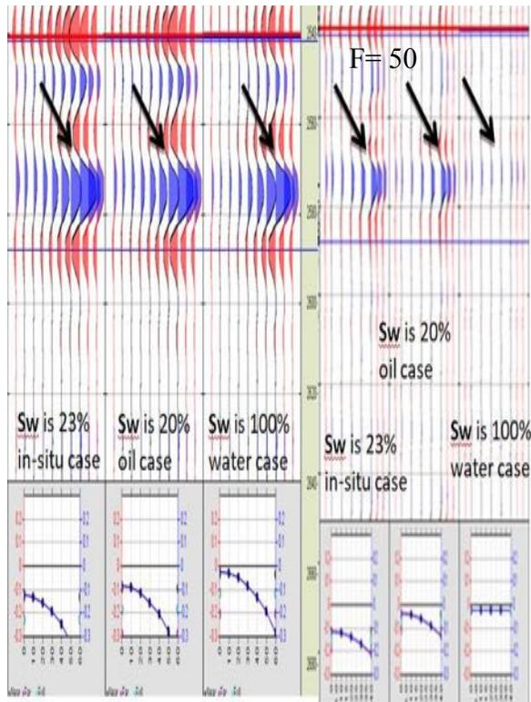
**Figure 6:** shows synthetic AVO modeling and fluid substitution for Yoyo-1 reservoir, one with ricker wavelet of 50 Hz, and the other of 70 Hz of three cases (in-situ case, gas case, and oil case).
