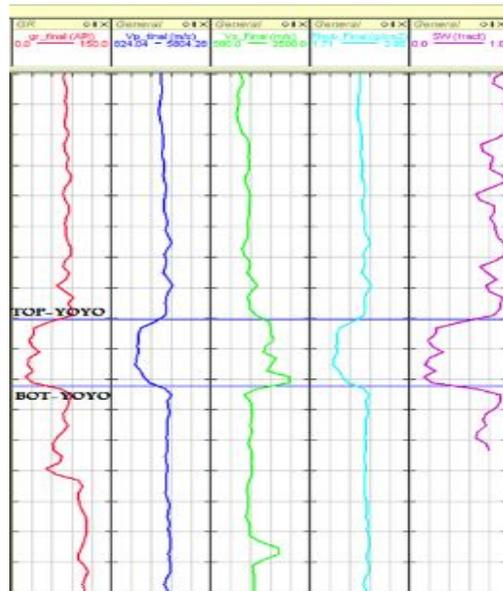
**Figure 4:** Illustrates the elastic parameters logs with  $S_w$ , and porosity log for Yoyo-1 reservoir.
