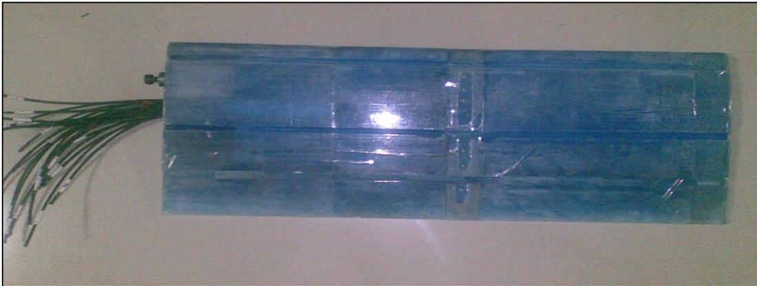
**Fig 2: The real model of NACA0015 airfoil**
