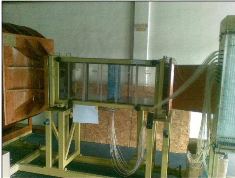
**Fig 4: Shows the blade inside wind tunnel**
