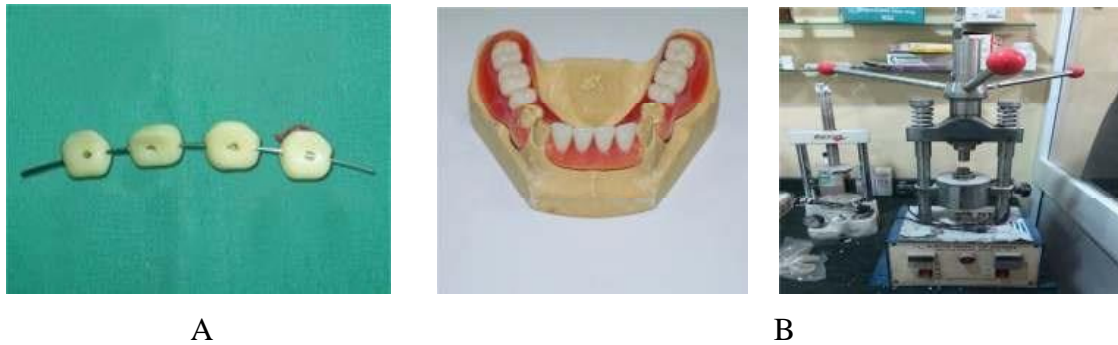
Figure 3. A- Shows the wire orientation of the holes. B- Manual compression unit used to ensure complete material flows through the sprues into the mold
