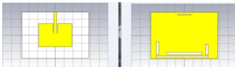
Fig. 4. Single Microstrip patch antenna with slots in ground plane.
