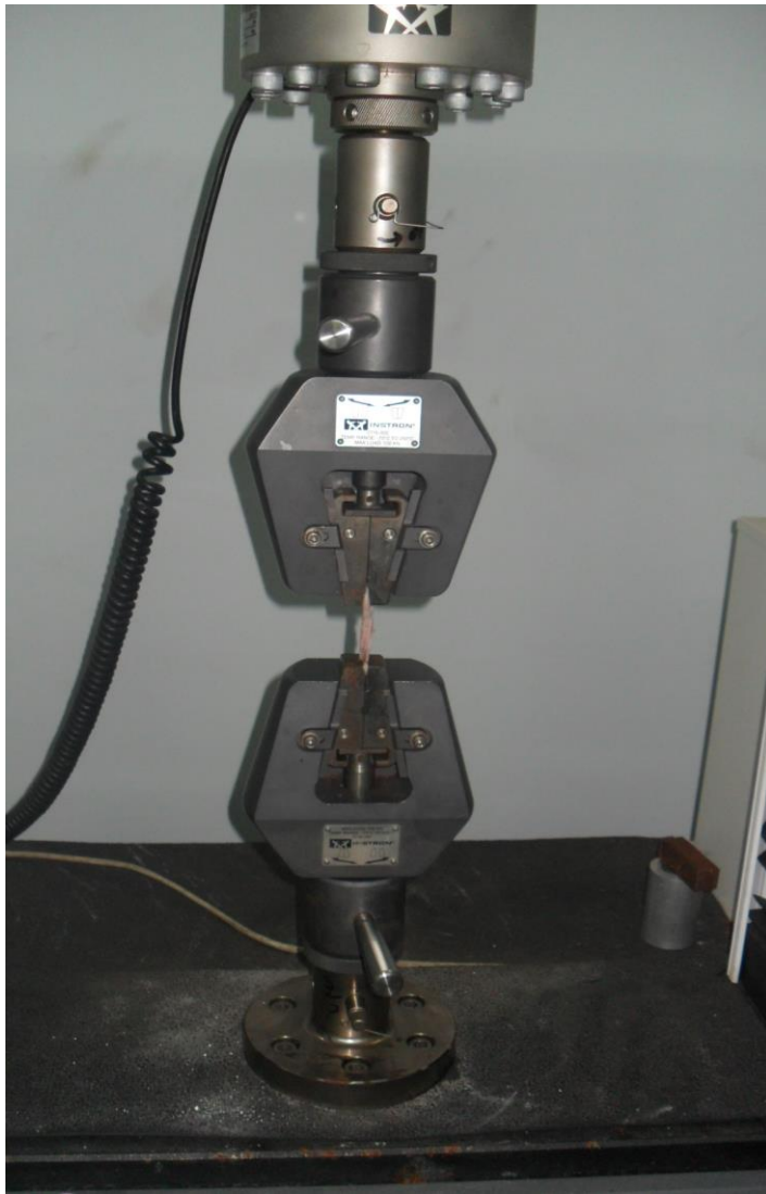
Fig. 6 shows the sample held in the tensile test machine.
