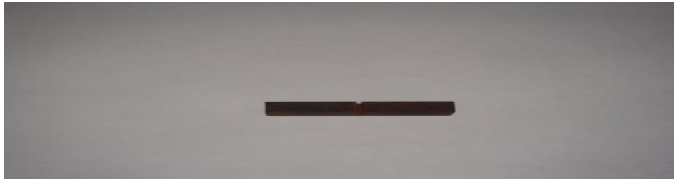
Fig. 1a: specimen for impact test
