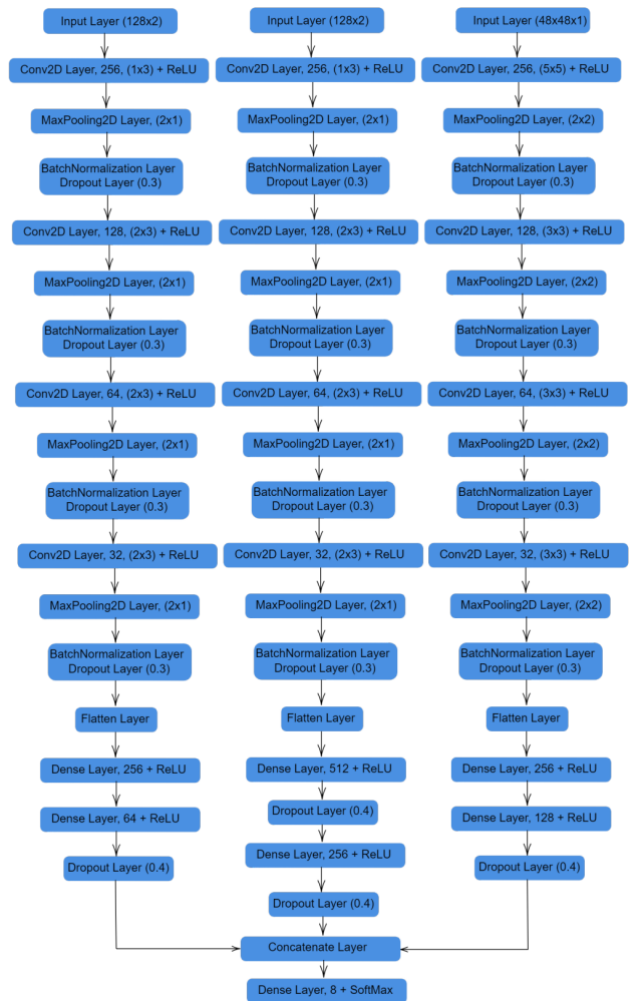
Figure 7: CNN-(IQ/AP/CD) Model Architecture. accuracy is plotted against various SNRs. The Training was carried out using Microsoft Azure and evaluation was carried out using Visual Studio Code environment. The code was written in python language.
