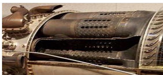
Figure. (9) Combustion Chamber
