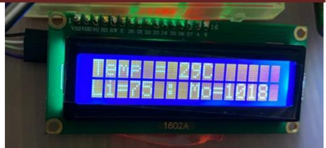
Fig.11. LCD displays the value of measured temperature, light intensity and soil moisture.
