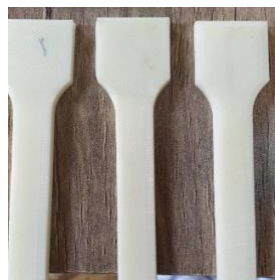
Figure 3b. Closed 3D printed specimens
