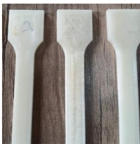
Figure 3a. open 3D printed specimens at room temperature
