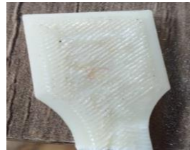
Figure 6d. open 3D printed surface roughness of specimens at room temperature
