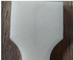
Figure 6c. Closed 3D printed surface roughness of specimens
