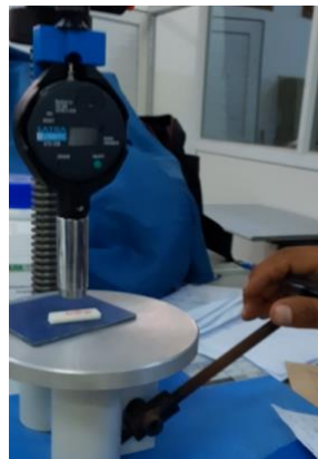
Fig.4. Hardness Test Machine
