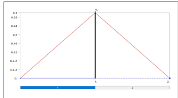
Figure 5: This graph shows the amount of displacement force applied to the balloon to expand the stent associated with time.
