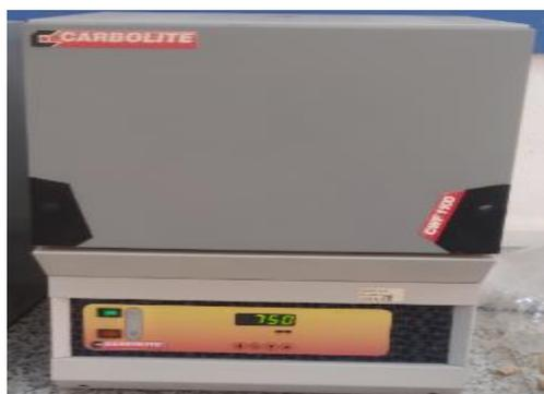
**Fig. 3 Zeolite activation at high temperature**
