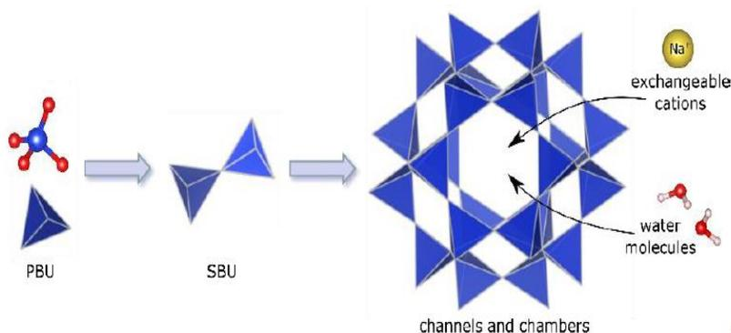
*Fig. 1 Scheme of Zeolite Structure[8]*
