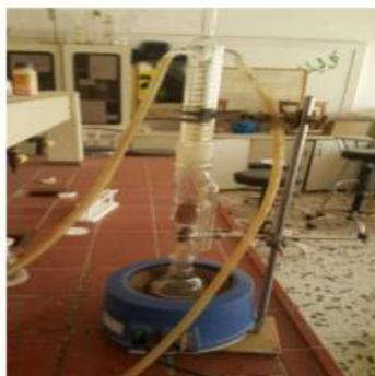
**Fig. 5** Soxhlet device used in core cleaning
