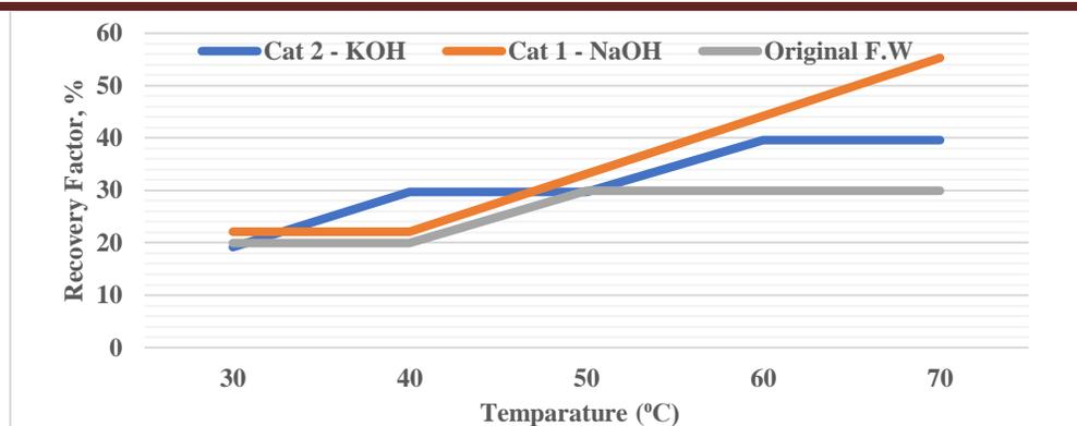
**Fig. 7 Comparison between recovery factors using different compositions of formation water**
