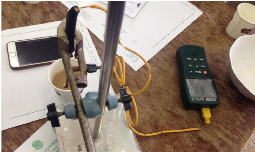
Figure 4. Photo of the setup consists of permanent magnet attached to thermocouple, Smartphone, plastic cup ice or hot liquid.
