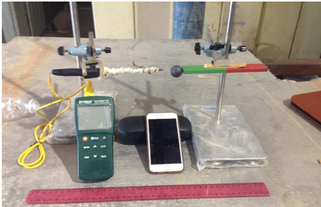
Figure 5. Photo of the experimental setup used to determine the Curie temperature of stainless steel spheres. The end of Type K thermocouple is inserted into a small hole in the sphere, the temperature of which is indicated.
