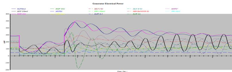
Fig.( 5.b). generator electrical power for a fault at (Khoms) of (2 sec.)
