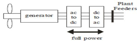
Figure (1): Variable Speed Wind Turbine Generator with Full Conversion Power Converter [2].
