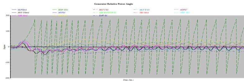
**Fig.(4.a) Relative Rotor angle for a fault at (Khoms) of (1.3 sec.)**
