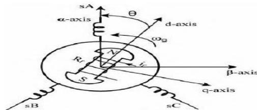
Figure (2) shows the DQ reference frame model used in a salient -pole synchronous machine[2].
