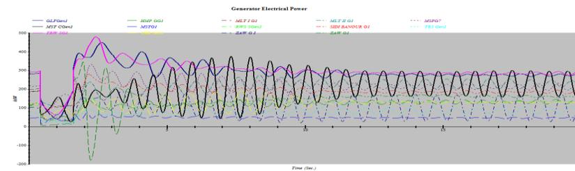
**Fig.(3. b) generator electrical power for a fault at (Khoms) of (1.2 sec.).**
