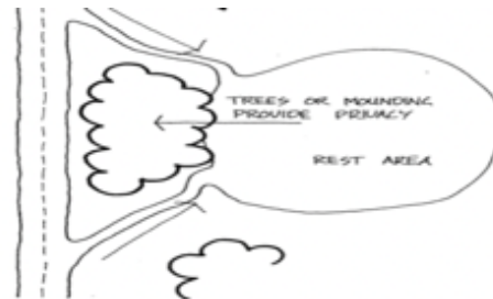
Buffer zone between the road and the restroom
