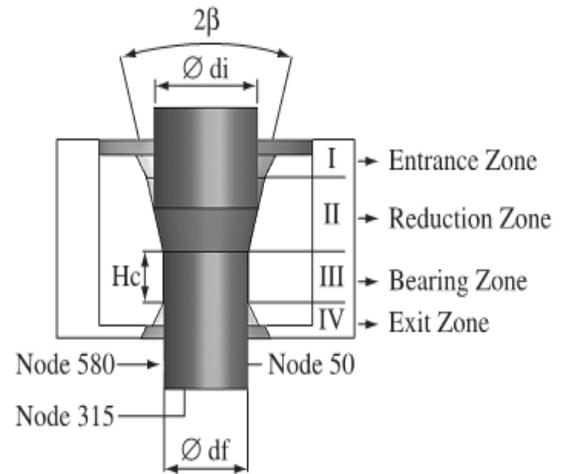
Fig.4. Scheme of internal die geometry, Source [11]
