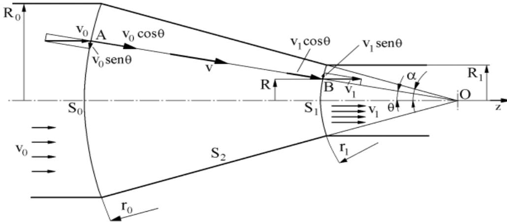
**Fig. 3. Velocity field assumed in Avitzur's theoretical model of drawing wire process; Source [30]**
