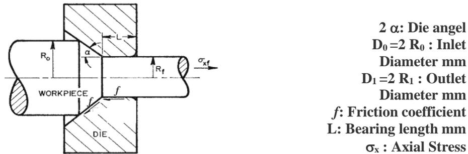
**Fig.2. described the schematic-pertinent parameters of a wire drawing process.**
