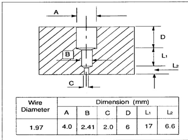
Hydrodynamic die for ø1.97mm mild-steel wire
