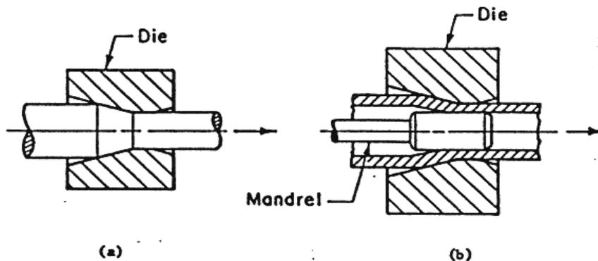
**Fig.1 Drawing process of (a) rod or wire & (b) tube or hollow, Source [3]**
