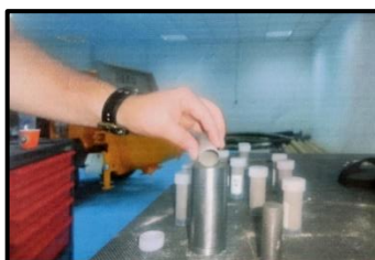
Fig. 1 illustrates the composite powders poured in the die.
