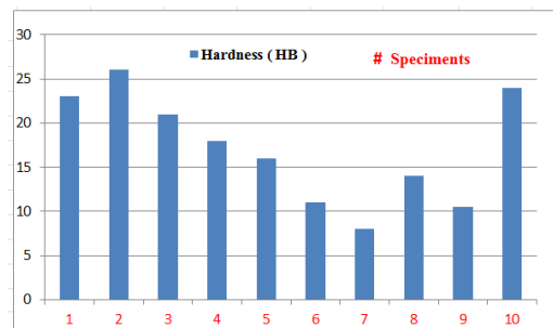
Fig. 11 Illustrates the hardness test result for all specimens of all (Fe-Cu 2 O-Al 2 O 3 ) compacted powers.
