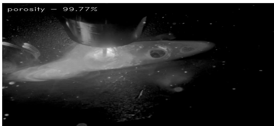
Figure. 3 weld porosity recognition model
