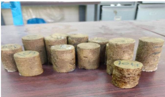
Fig. 13. Core Sample After Sea Water Injection
