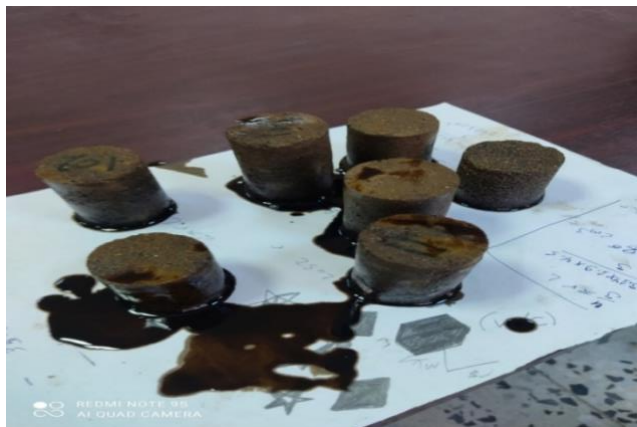
Fig. 11. Saturated Sample with Crude Oil
