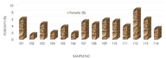
Fig. 14. Porosity for Each Core Sample
