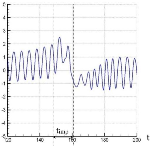
Fig. 10. Lift force coefficient for  $r_{\max}=2.0$
