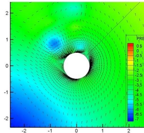
Fig. 5. Close-up view for wind flow around the cylinder
