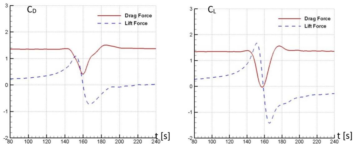
**Fig. 12, 13.** Mean values of drag and lift force coefficients for  $r_{\max}=2.0$  (left) and  $r_{\max}=4.0$  (right)
