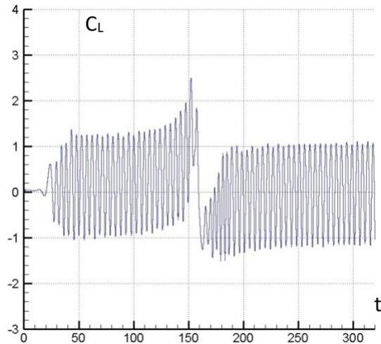
Fig. 7. Lift force coefficient for  $r_{\max}=3.0$
