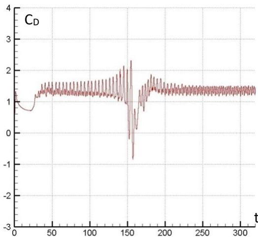
Fig. 6. Drag force coefficient for  $r_{\max}=3.0$
