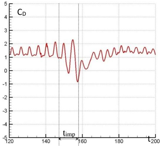
Fig 8. Drag force coefficient for  $r_{\max}=2.0$
