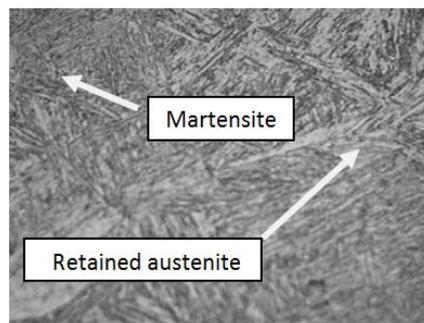
**Fig. 10: Micrograph of martensitic AISI410 austenitized at 1010°C, consists of retained austenite and martensite matrix with no visible carbides. The hardness is 36.5HRC. Magnification of 200X.**
