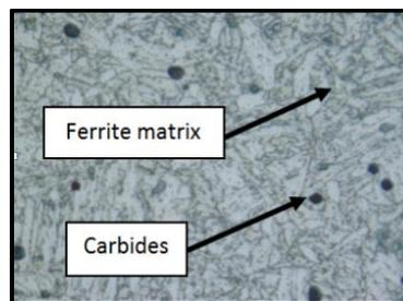
**Fig. 5: Optical photomicrograph of AISI410 in the annealed form.**
