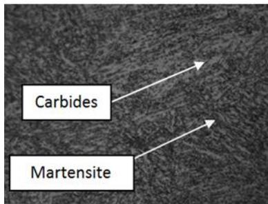
**Fig. 7: Photomicrograph of AISI410 austenitized at 925°C, quenched and tempered at 260°C shows Martensite with fine-carbides precipitates. The hardness is 38.5HRC.**
