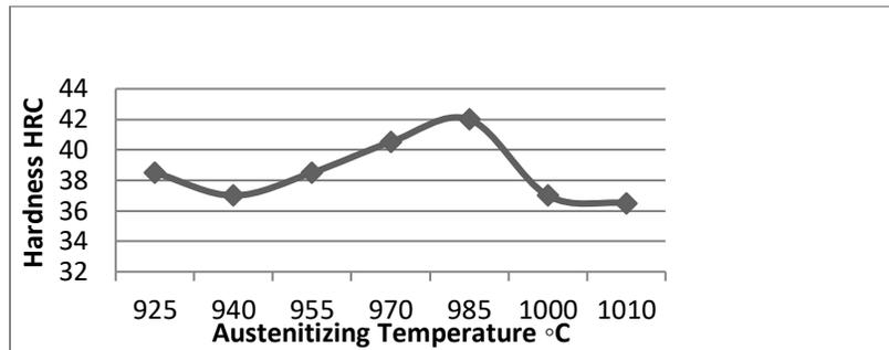
**Fig. 3: The influence of varying austenitizing temperatures on the hardness of martensitic AISI410 Type.**
