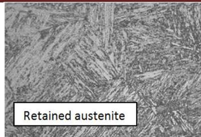
**Fig. 9: Photomicrograph of AISI410 austenitized at 985°C.**
