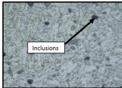
**Fig. 6: Optical photomicrograph of AISI410 sample in the annealed form showing the defects. Magnification of 200X**
