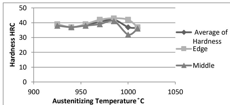
**Fig. 4: The influence of varying austenitizing temperatures on the hardness at different regions of martensitic AISI410 samples,**
