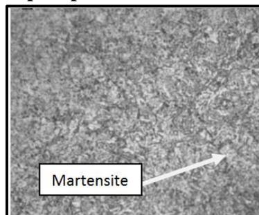
**Fig. 8: Photomicrograph of AISI410 austenitized at 955°C, shows fine martensitic matrix with less undissolved carbides. The hardness is 38.5HRC. Magnification of 200X.**
