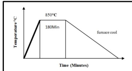
**Fig. 1: Heat Cycle of annealing process.**
