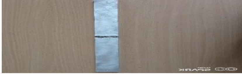
Fig. 5: specimen of welded aluminum alloy 5052
